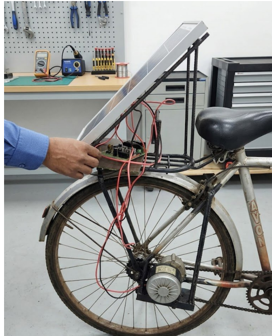
Fig. Electric Motor Installation on the Rear Wheel Hub
